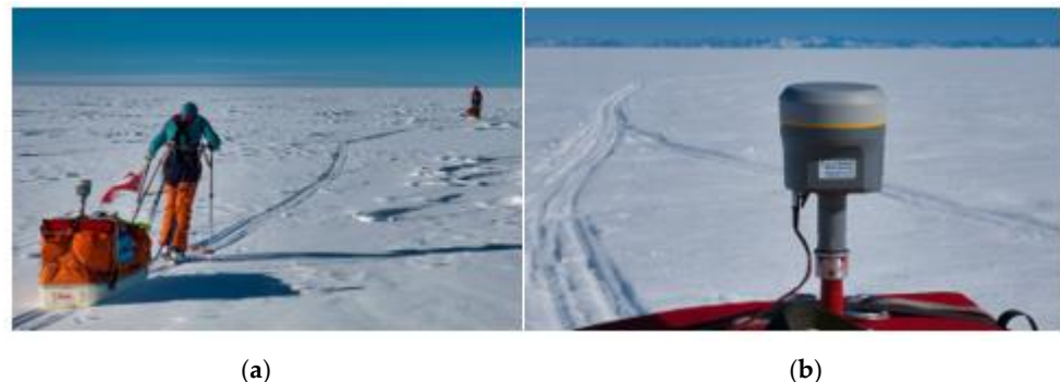
Figure 4. Kinematic GNSS measurement during GKE 2020 (a) on the pulka. (b) Trimble R12.
